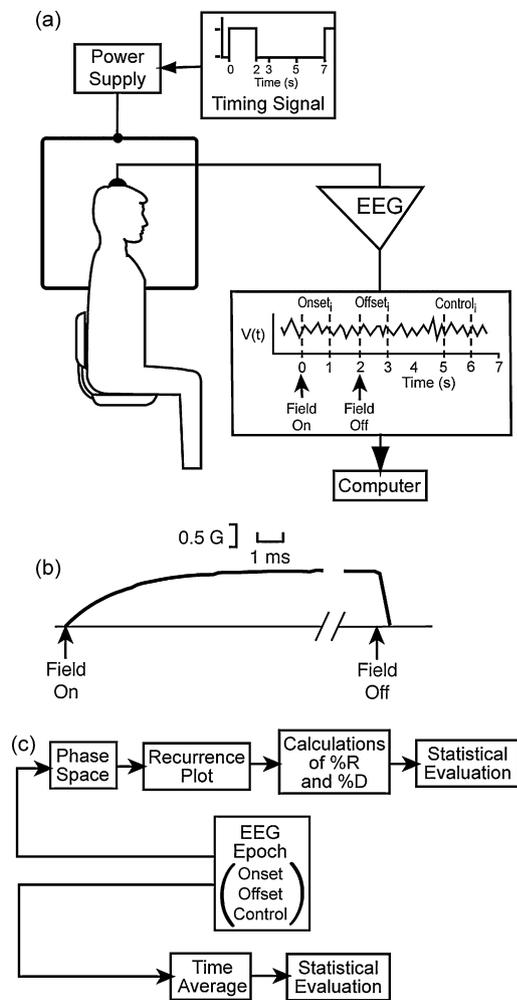
**Fig. 3.** Application of magnetic fields. (a) Schematic diagram of the exposure and EEG-detection systems (mid-sagittal view). (b) Onset and offset of the magnetic field. (c) Procedures for nonlinear and linear analysis.
