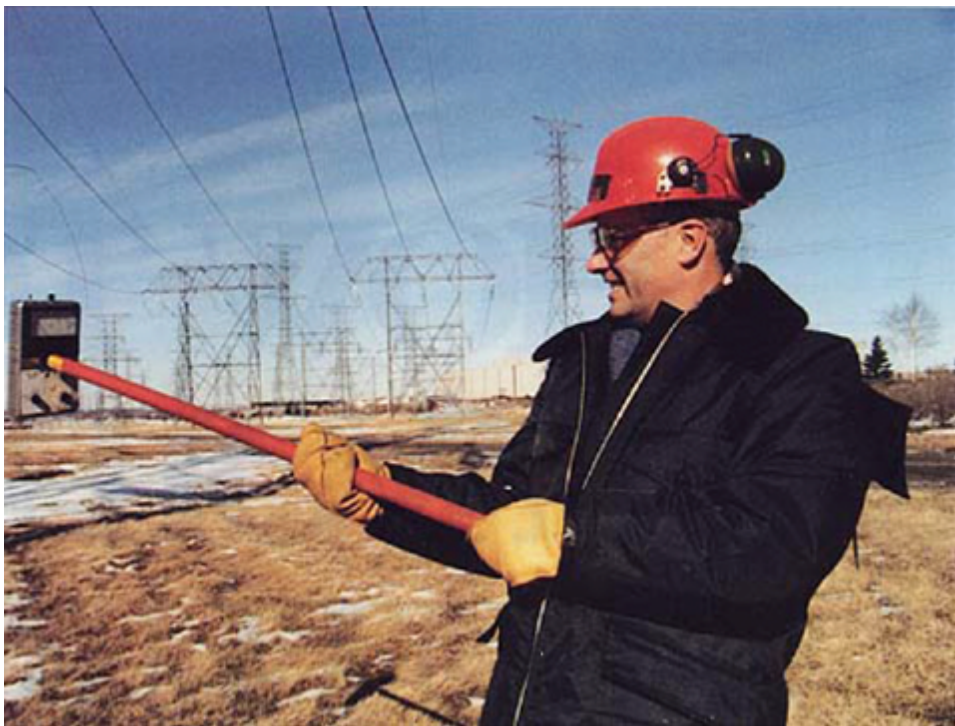
A technician measures electrical field strength beneath a transmission line near Toronto, Ontario. Photo by Ontario Hydro
