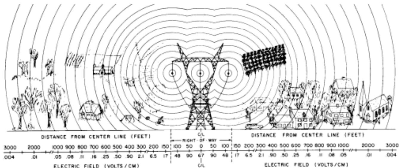
**Figure 2.** A 765 kV transmission line such as proposed by the Rochester Gas and Electric Corporation, Rochester, New York, illustrating the existence of the electrical energy which is being transported by the line. The energy is transported continuously and much of it moves through space in a region beyond the right-of-way. The energy is composed of an electric and magnetic field. For simplicity, only the electric field magnitude is shown at each lateral distance.
