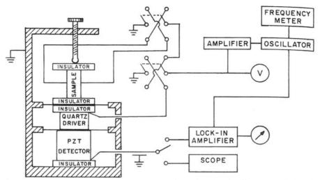
Fig. 1. Apparatus employed in the measurement of the piezoelectric effect.  $V_8$  applied to the sample causes a deformation by virtue of the converse piezoelectric effect. It is transmitted to the quartz detector which produces an output voltage  $V_{out}$  by means of the direct piezoelectric effect of quartz. With the switch reversed  $V_q$  is applied to the X-cut quartz driver so as to produce  $V_{out}$ . The apparent piezoelectric constant for the samples studied was then calculated as:
